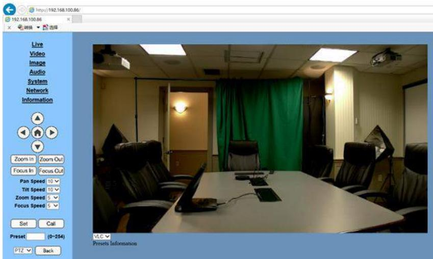
10. You should now be able to receive an RTSP stream from your camera. The following video, <https://www.youtube.com/watch?v=hmqI0hjTOUI&feature=youtu.be>, shows how to setup an RTSP stream in Wirecast as an example. You'll see how to use ONVIF to easily set up two (2) PTZOptics cameras with Wirecast, note that the ONVIF feature must be enabled in the "Network" settings for ONVIF discovery to work properly.
