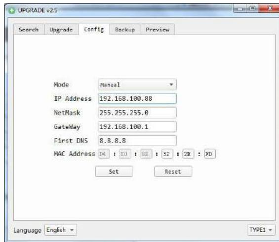
(Note that in more complex network environments you may have to request a “Static IP” from the IT department to prevent any possible network complications in addition to the “Static IP” you will likely need an appropriate Network Mask, Default Gateway and First DNS)
